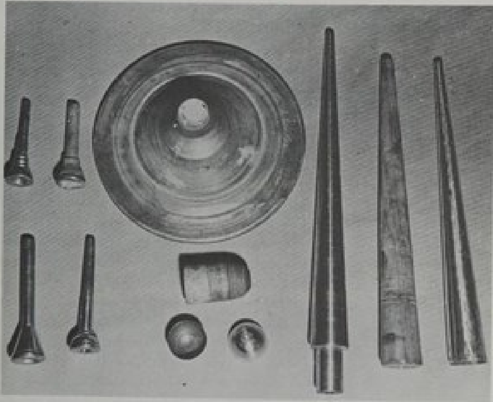
FIGURE 35. Brass instrument tools and parts: left , mouthpieces and a rough mouthpiece casting; center , forms for spinning bell and ball; right , steel and wooden mandrels and a seamed cone.
