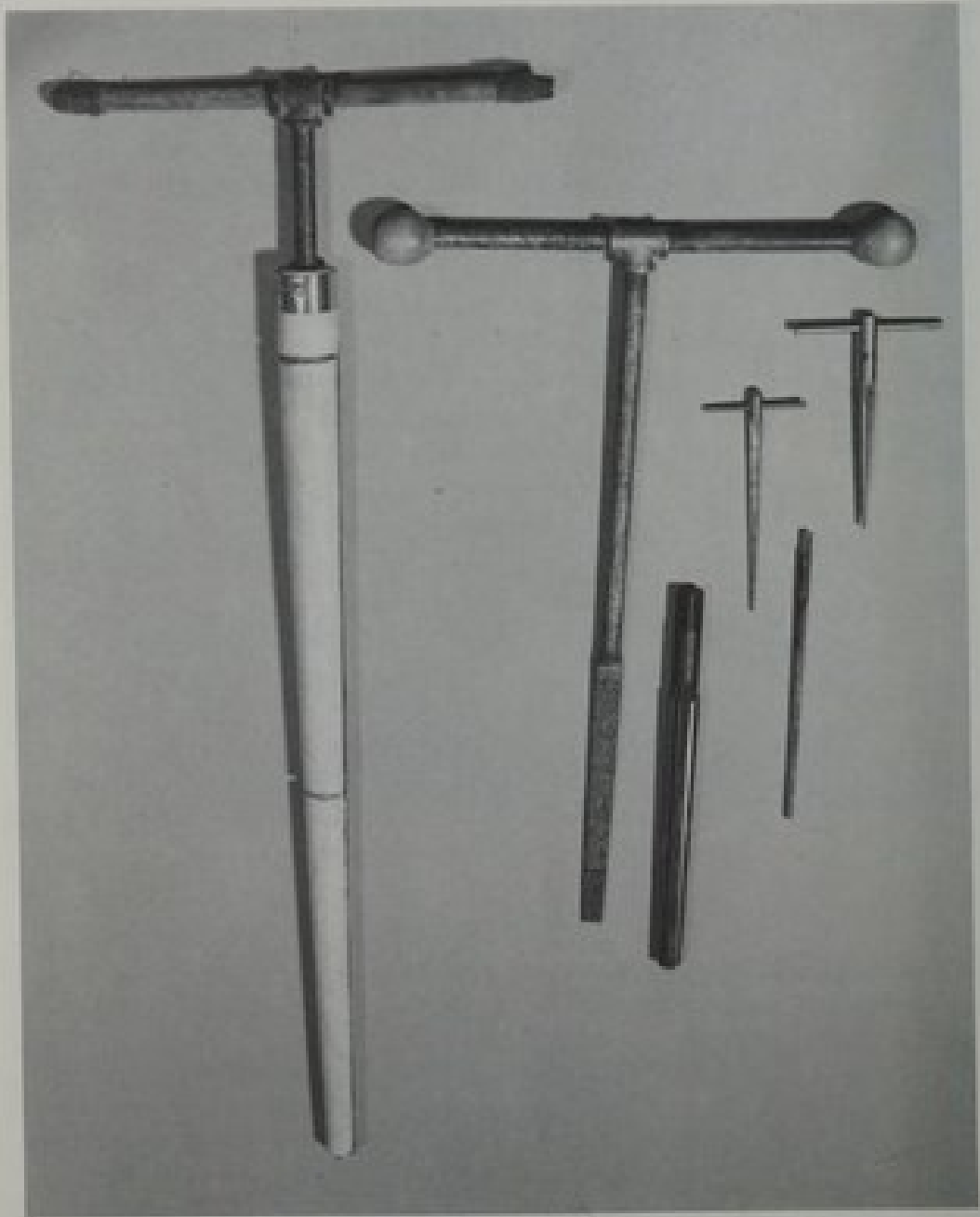
FIGURE 3. Left , four steel-fluted reamers; center , flat reamer ground from file; right , wooden bodied reamer.
